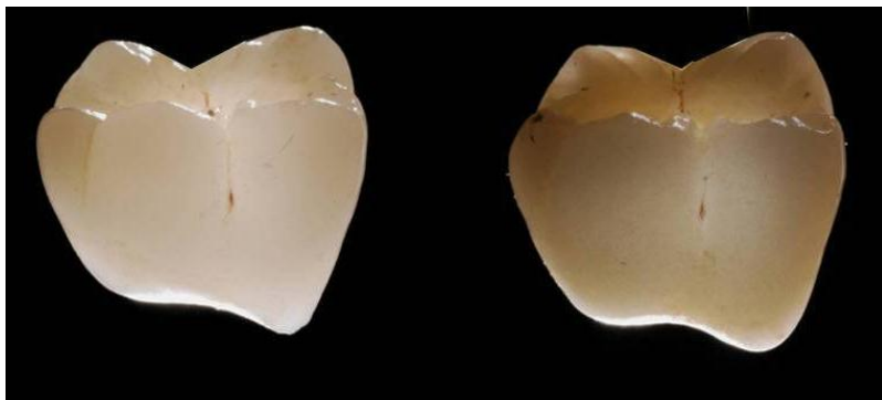
Figure 2: Translucency of lithium disilicate (LS2) and zirconium oxide (ZrO2) ceramic in transmitted light
