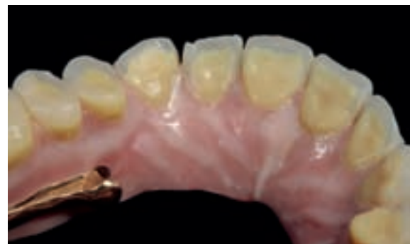
Fig 1 Removable implant-borne bar-latch prosthesis with conventional PMMA denture teeth after a service life of two years. High chewing forces and poor wear properties resulted in the rapid damage of the occlusal surfaces.
