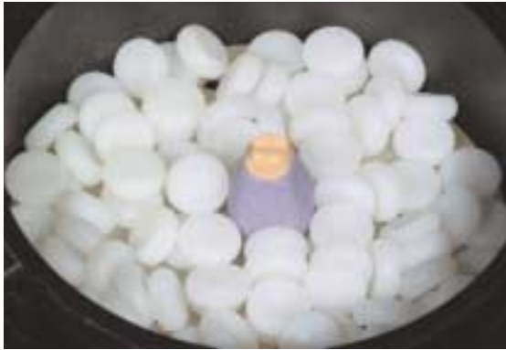
Position the die in the Vectris VS1 unit; apply a small amount of Vectris Glue to the die.
