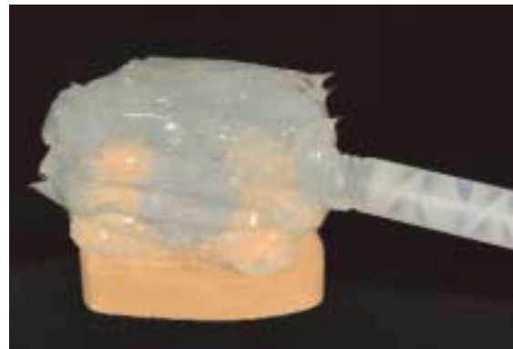
Apply a thin coating of Vaseline to the laboratory silicone and then apply Transil.
