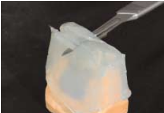
Smooth out the exterior surface of the Transil matrix and form it into a conical shape.
