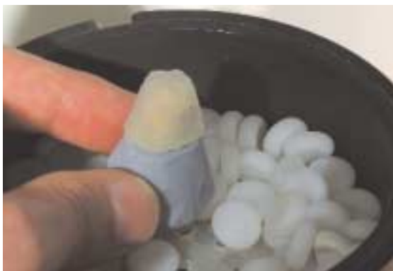
Position the die with the Transil matrix in the VS1. Start the vacuum-forming and polymerization process. The program takes 10 minutes to complete.
