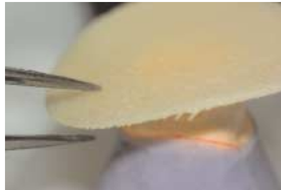
Remove the Vectris Single from the light-protected package; place it on the die with tweezers and lightly press it into place.
