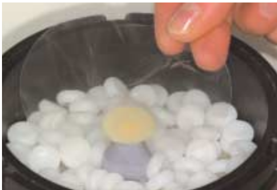
Cover with Vectris foil; start Program 1 for the vacuum-forming and polymerization process.
