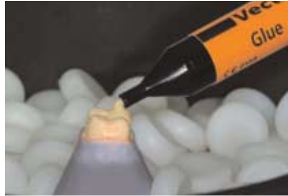
Position the die in the Vectris VS1 unit; apply a small amount of Vectris Glue to the die.
