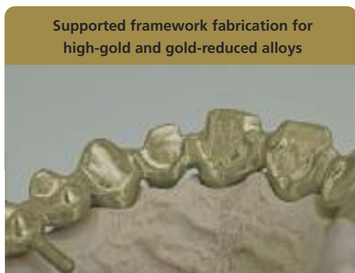
Fitting and inspection on the master model
