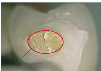
Incorrect cross-section of the metal-framework of 1.5 x 2.5 mm = 3.75 mm 2 – vertical dimension only 1.5 mm in the bending direction!
