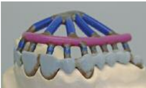
Wax framework sprued for conventional bar casting
