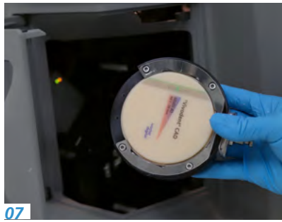
07 — The SR Vivodent CAD Multi disc is mounted with the labelling facing upwards
