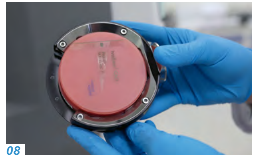
08 — The IvoBase CAD disc is mounted for the fabrication of the denture base
