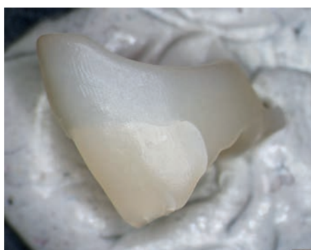
Fig. 3 The tooth shown on this image (NU5 Tooth 5) broke at a load significantly exceeding 1000 N (i.e. approx. 100 kg). Typically, the fracture occurred in the buccal area by large-scale chipping. If intrinsic tension had been present in the material, an even fracture pattern at a low load would have occurred.
