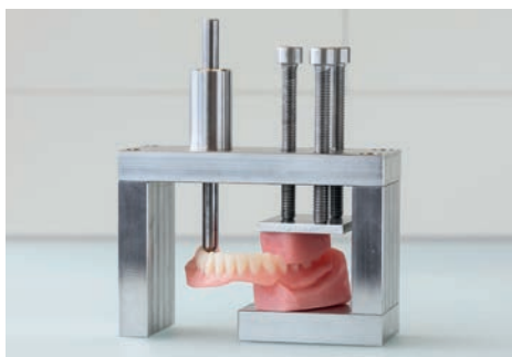
Fig. 11 Study setup for torsion loading The study setup depicted above shows a denture base body secured on one side with suitable clamps made from denture base material. Torsional forces were generated in conjunction with tooth 46 with the help of a rounded metal punch.
