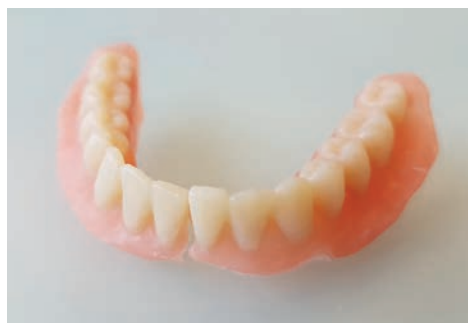
Fig. 12 Fractured test specimen consisting of two bonded tooth segments (31–37 and 41–47) after fracture testing. The samples fractured already at 70% of the loading threshold of the unsegmented dental arches (14 teeth) and they did so exactly in between the two bonded segments.
