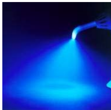
Fig. 19b: Light scattering of a very tapered light guide (13>8 mm)
