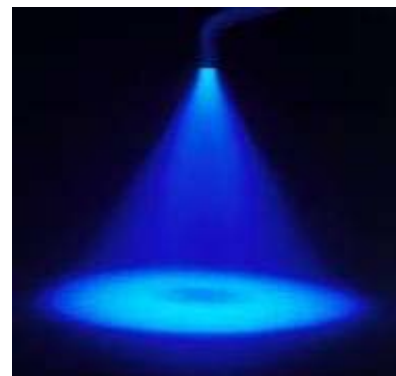
Fig. 19c: Homogeneous light scattering of a parallel light guide
