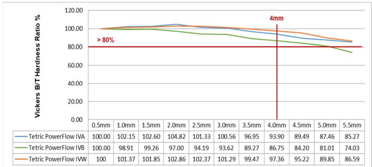
Fig. 43: Bottom/top Vickers hardness ratios at 0.5mm intervals for each of the Tetric PowerFlow shades
