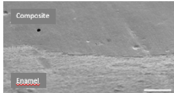
Figs. 41a-b: Comparison of continuous margins in enamel of Tetric PowerFill according to different etch techniques. SEM 200x, Bar = 100µm
