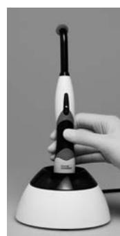
Since the battery is an expendable part, it has to be replaced after its typical life cycle has expired after approximately 2.5 years. See battery label for the age of the battery.
