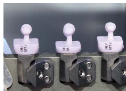
11 — Completed, milled crown made of IPS e.max CAD MT blocks in the CAD/CAM milling machine
