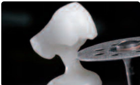
The sprues are cut with a fine diamond disk.
