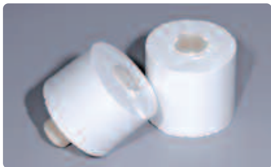
Separate the investment ring using a separating disk and break it at the predetermined breaking point.
