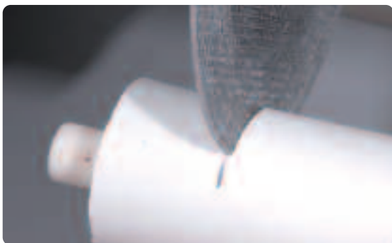
Separate the investment ring using a separating disk and break it at the predetermined breaking point.
