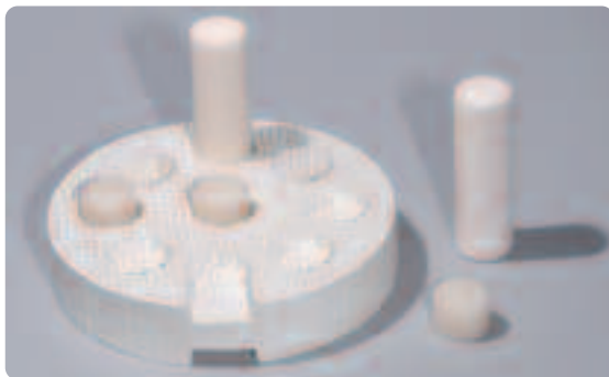
Position the IPS Empress Esthetic ingots and AIOx plungers on the IPS UniTray.
