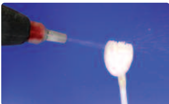
Blast the restoration with \text{Al}_2\text{O}_3 (Type 100) at 0.5 bar pressure.
