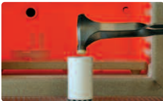
Place the hot IPS Empress Esthetic ingot in the investment ring.
