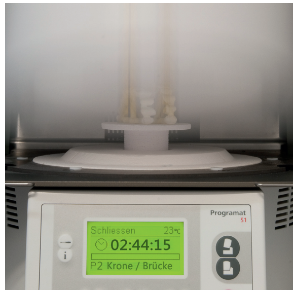
Fig 15 During the closing of the furnace chamber, the remaining sinter time of less than 180 minutes is displayed.
