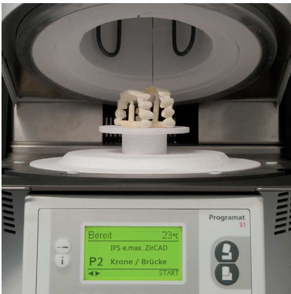
Fig 14 The frameworks are sintered in a vertical position on the sinter tray without a bead bed.
