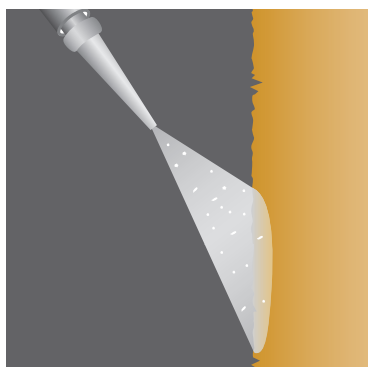
Correct angle to blast alloy surface
