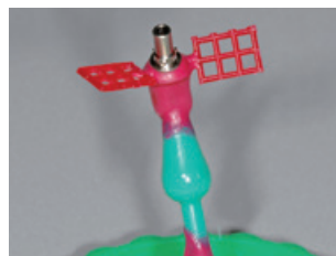
Sprued abutment with cooling fans
