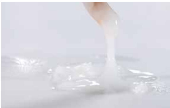
If mixed correctly, the consistency of the glazing material must not be too liquid.
