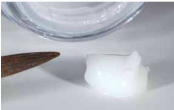
Mix the IPS Ivocolor Glaze Paste with an agate spatula before removing it from the jar.
