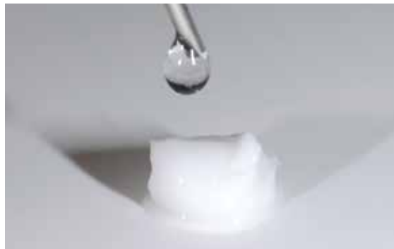
Mixing of the IPS Ivocolor Glaze paste with IPS Ivocolor Mixing Liquid allround or longlife
