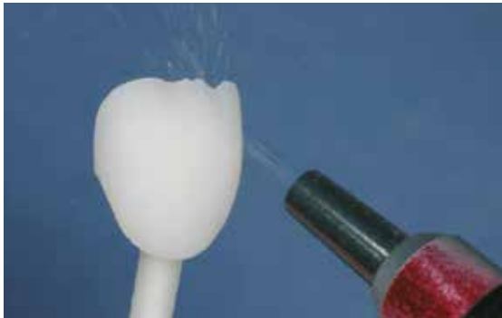
Carefully blast the restoration with \text{Al}_2\text{O}_3 at 0.5 bar pressure (Caution: abrasive).
