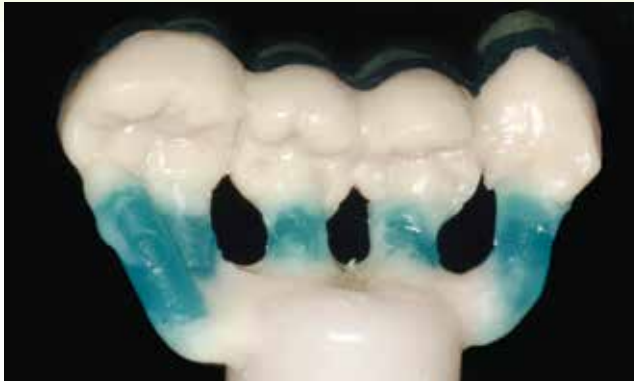
Fig. 18 Spruing on the investment ring
