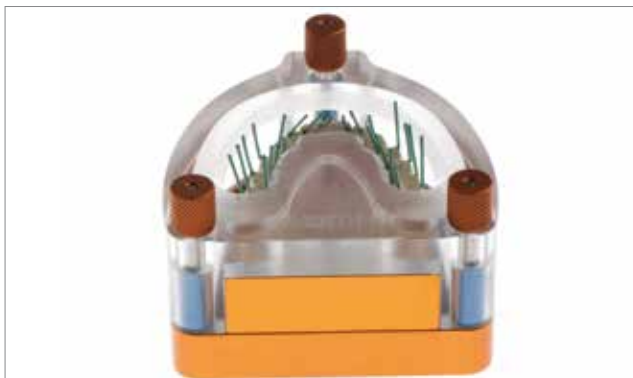
Fig. 3a and b The mock-up was duplicated in a transparent flask using clear silicone material.
