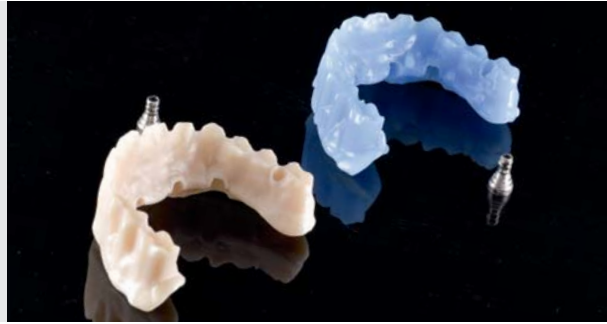
Fig. 5: Comparison between the wax structure and the sintered framework
