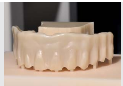
Fig. 3: Sintering the framework. Small sinter drops support the framework during sintering.
