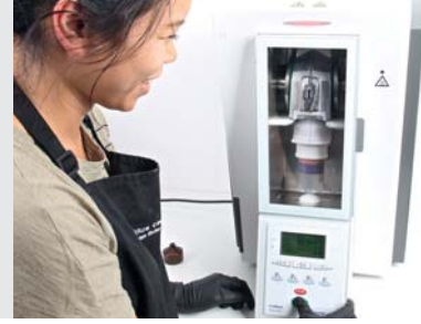
Fig. 6: The flask and IvoBase mixture are placed in the injector and the program is started.
