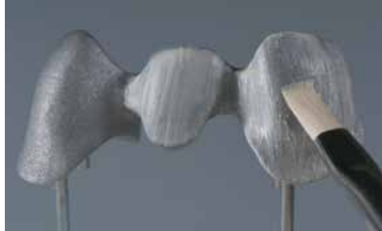
Application of IPS Style Ceram Paste Opaquer
