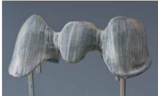
IPS Style Ceram Paste Opaquer after the 1 st Opaquer firing
