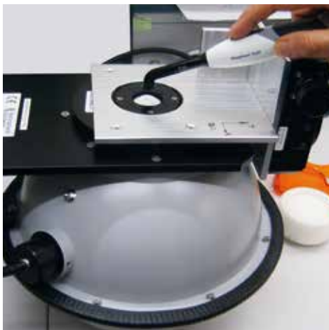
Fig. 5 Test setup with integrating sphere
