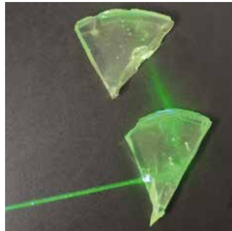
Fig. 3 In this sample, the laser beam is bent on entering and leaving the material.
