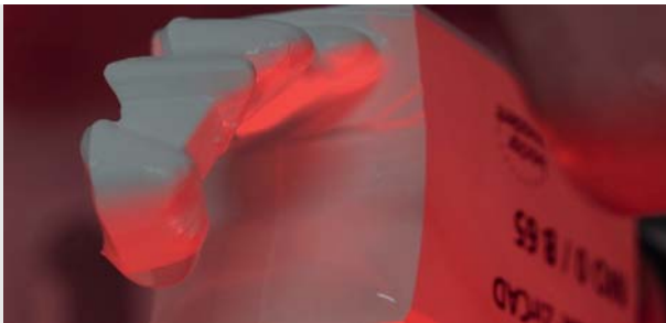
Fig. 8: Zirconium oxide framework in the process of being milled
