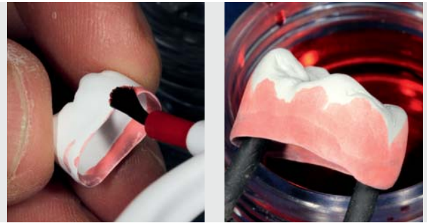
Figs 10a and b: Brush infiltration before sintering: The colouring liquid is applied in the cervical areas.
