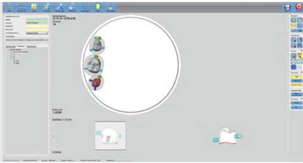
Fig. 7: Same digital data set: preparation for the fabrication of the zirconium oxide crowns (Zenostar Zr Translucent) with CAD/CAM equipment
