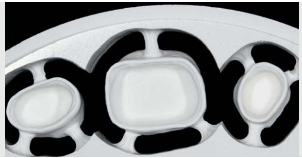
Fig. 8: The milled crowns before they were trimmed from the zirconium oxide disc
