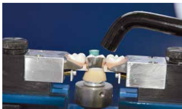
Fig. 8: Oblique position of the light probe and 5-mm distance to the tooth
