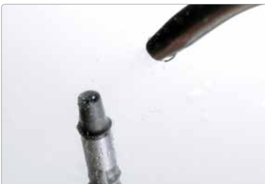
Remove silicone and subsequently clean in an ultrasonic bath or with the steam jet.
