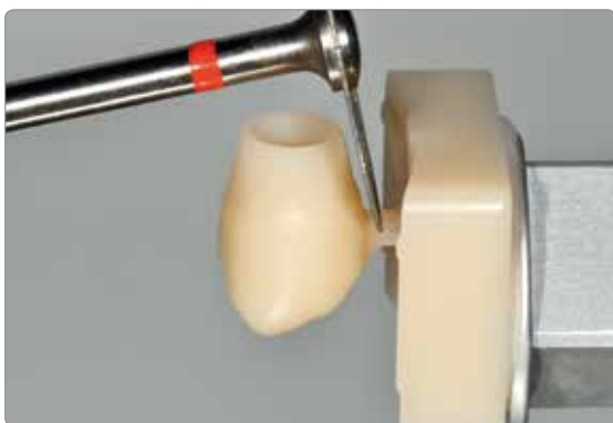
Separate the attachment point from the incisal using a fine, cross-cut bur or a diamond separating disc.
