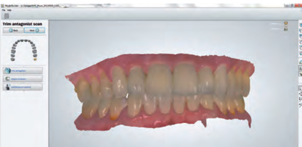
Fig. 4 Digital scans of the temporaries (3Shape Trios Color) served as a "mock-up" of the final restoration.
