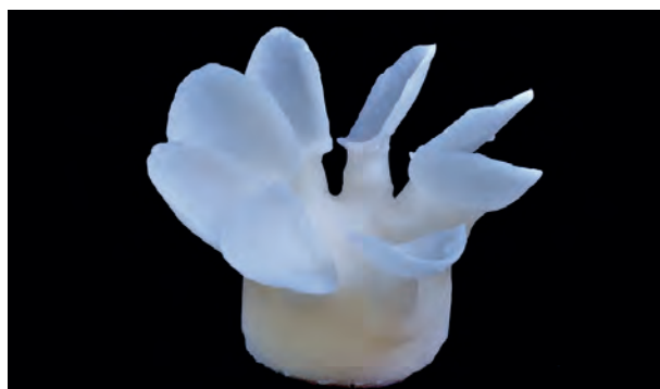
Fig. 4 The pressed frameworks (IPS e.max Press LT) were approximately 0.3 mm thick. We took advantage of the light-optical properties of the translucent ingots (Low Translucency).
