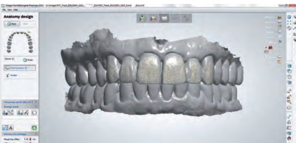
Fig. 6 Colours in the design software indicate differences between the final crown design and the temporaries (proposed crown design: yellow; pre-preparation scan: grey).
