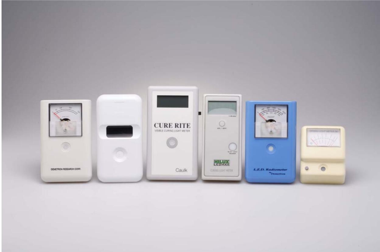
*Fig. 8: Different commercial radiometers*
