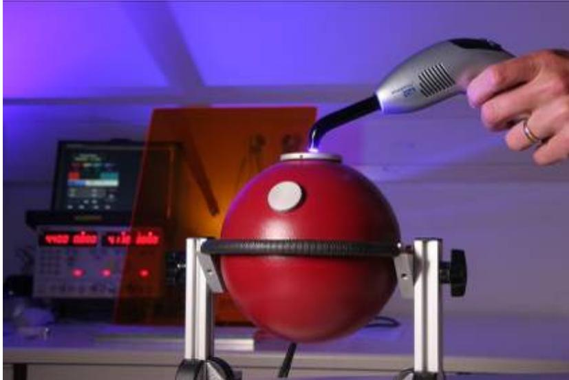
*Fig. 9: Measurement with the integrating sphere*
