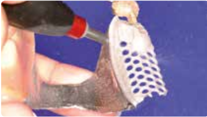
Blast with Type 100 Al_2O_3 at 2–4 bar / 29–58 psi pressure.
