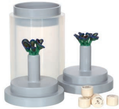
Fig. 8 Single frameworks were waxed up, invested and pressed using IPS e.max Press MO ingots.
