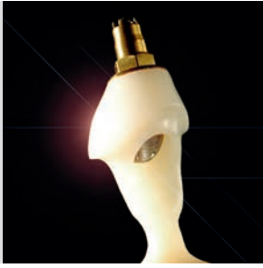
Fig. 6 The IPS e.max Press abutment on the titanium base (coated with titanium nitride) after divestment
