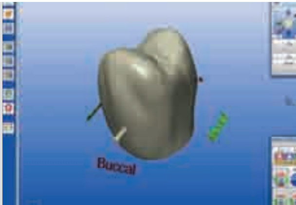
Fig. 5 Virtual design of the crown. The picture illustrates the “modeling” of the temporary restoration on the computer screen using the CEREC Biogeneric software.
