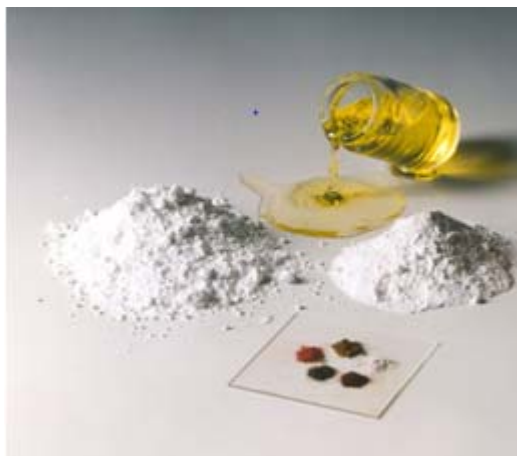
Fig. 1: Components of a typical composite: monomer mixture, fillers, initiators, catalysts and pigments.
