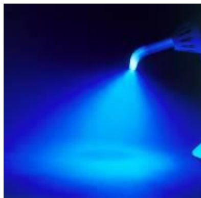
Fig. 8b: Light scattering of a very tapered light guide (13 > 8 mm)
