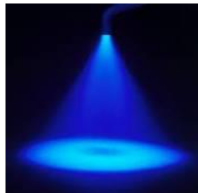
Fig. 8c: Homogeneous light scattering of a parallel light guide
