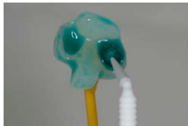
Apply the self-etching Monobond Etch & Prime to the bonding surface using a microbrush and scrub it into the surface for 20 seconds. Allow to react for another 40 seconds.
