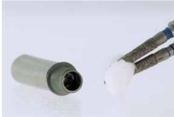
Seal the screw channel with a foam pellet or wax. Make sure that the bonding surface is not contaminated.
