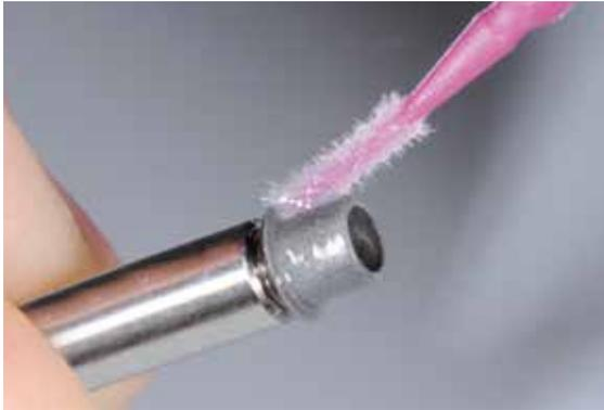
Apply Monobond Plus on the cleaned bonding surface and allow to react for 60 seconds. After the reaction time, dry the remaining residue with water- and oil-free air.
