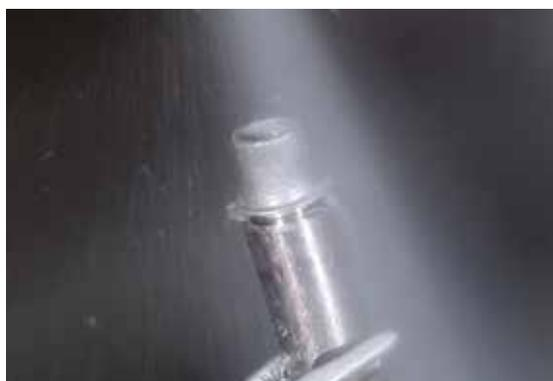
Clean with an instrument and steam cleaner. Make sure that any wax residue is carefully removed.
