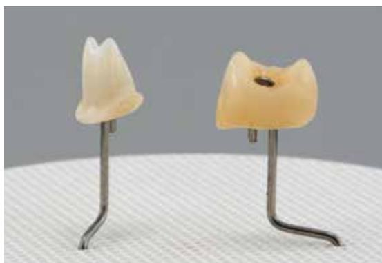
Conduct Stain firing on a honey-comb tray suitable for the ceramic furnace.
