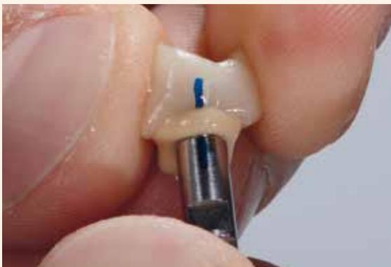
The titanium bonding base is introduced into the ceramic structure. In doing so, the alignment of the two components is checked (rotation lock/marking). The components are firmly held in place for approx. 2:30 minutes until the Virtual Extra Light Body Fast Set has set.
