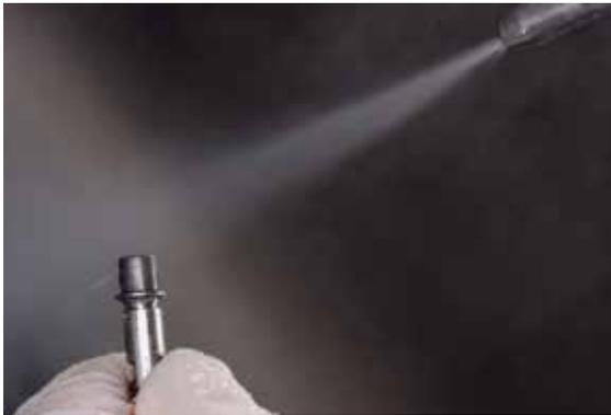
Clean in an ultrasonic bath or with a steam cleaner and then dry with blown air.
